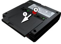
→ Press the battery cover on the underside of the unit ① lightly and push the battery cover in the direction of the arrow.
