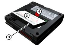
→ Lift the battery (2) by the tab (3). → Remove the slide (4) from the device.
