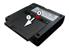
→ Press the battery cover on the underside of the unit 1 lightly and push the battery cover in the direction of the arrow.
