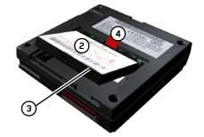
→ Lift the battery ② by the tab ③.→ Remove the slide ④ from the device.
