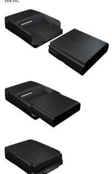
When inserting the Becker® MAP PILOT make sure that it is pushed in until it stops.
